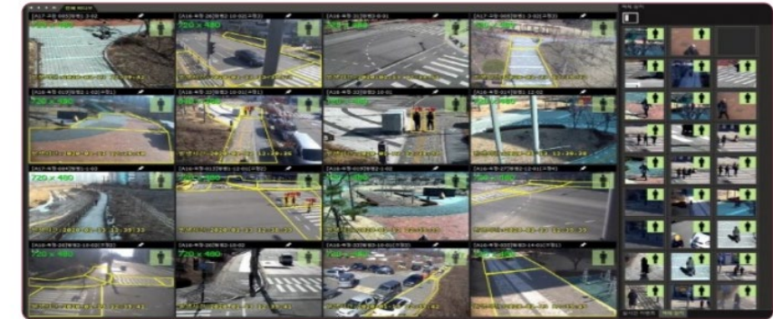
▲ The system analyzes CCTV footage, recognizing and categorizing spaces, objects, and individuals.
